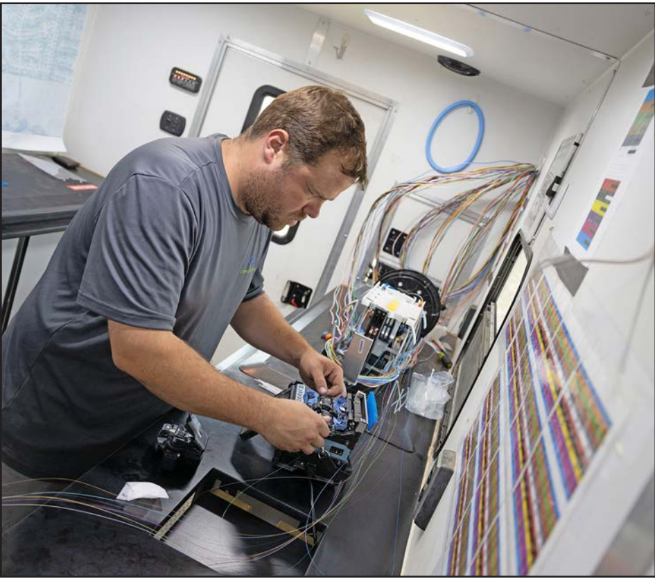
Working from a trailer, a Great Plains Communications technician joins two fiber optic cables together in what is called fiber splicing in this image provided by GPC. Crews will begin working in Arnold soon to bring fiber to in-town residents.
